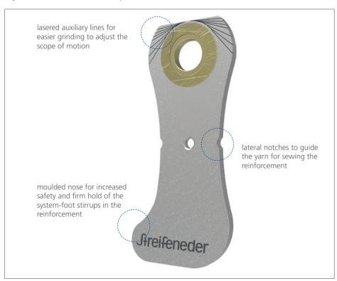
The Artikon.malleo system-foot stirrups form the second moving part of the ankle joint and are constructed in two different types - for rivet and lamination technology.
