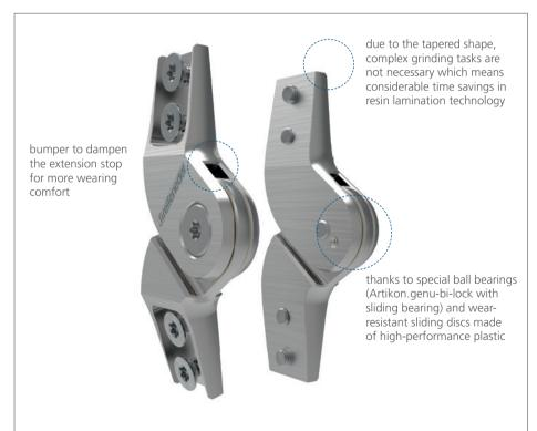
The monocentric system-knee joints Artikon. genu are intended for bilateral movement guidance and support of the human knee joint. Since the joints in the pivot point are relocated back to the rail, the rails can be optimally positioned on the upper and lower legs. The joints without lock, Artikon.genu, are also available in tapered form. Thanks to their narrow design at the ends, these can be used directly in the moulding method. The time-consuming grinding of the joints is no longer necessary.
