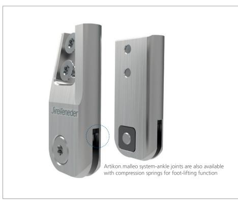
The Artikon.malleo system-ankle joints are freely moving and are used for bilateral motion control. If a foot-lifting function is desired, special ankle joints with compression springs are available. These support dorsal extension in the upper ankle joint, thereby causing a dynamic lifting of the foot during the swing phase.
