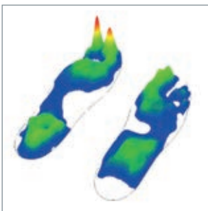
Foot pressure measurement: left daytime shoe, right Mars
