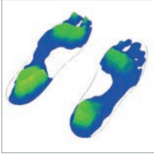
Foot pressure measurement: left daytime shoe, right Sirius
