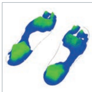
Foot pressure measurement: left daytime shoe, right Merkur A
