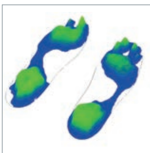
Foot pressure measurement: left daytime shoe, right Komet
