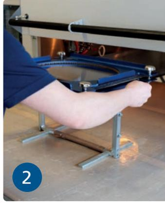
2 Prepare the thermoforming material and heat to processing temperature.
