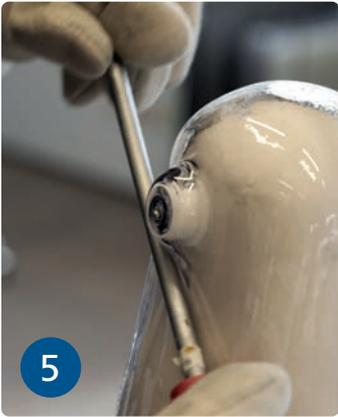
5 Reshape the edges of the dummy with a round object.
