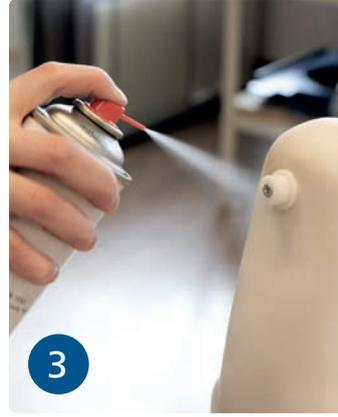
3 The model and dummy must be insulated to facilitate demoulding.
