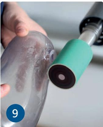
9 Sand the socket to the height of the mark on the dummy.
