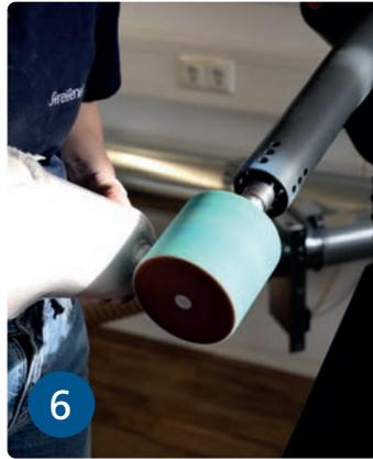
6 Sand the dummy down to the screw.
