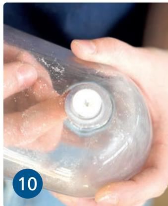
10 Check the grinding with the dummy, making sure that the grinding surface is flat.
