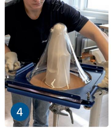
4 Deep-draw the heated material over the plaster model and dummy.
